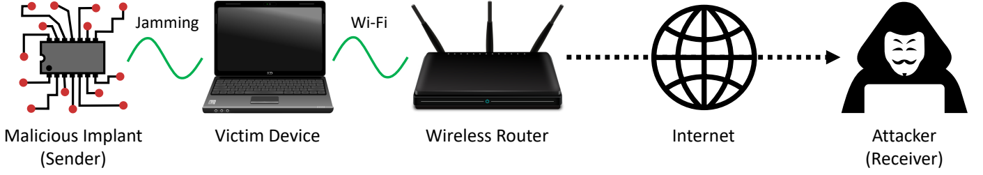
Figure 4: The general Wi-Fi Micro-jamming attack model.
