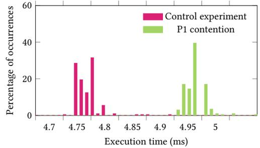
Figure 3: Port 1 contention experiment on `i64.ctz` for 1 000 000 instructions.
