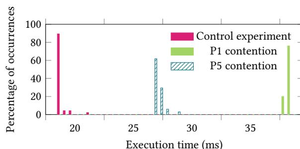
Figure 9: P1 contention experiment on `i64.rem_u` for 1 000 000 instructions.
