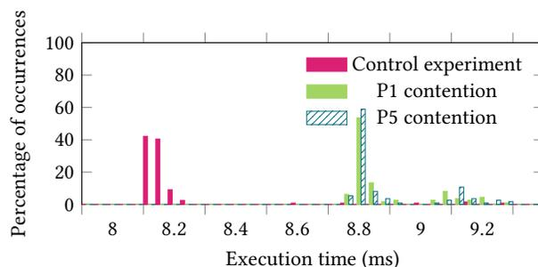
Figure 8: P1 contention experiment on `f64.floor` for 1 000 000 instructions.
