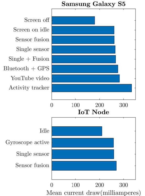
Figure 4: The effect of enabling SDI on the instantaneous power consumption of a smartphone (top) and an IoT node (bottom)
